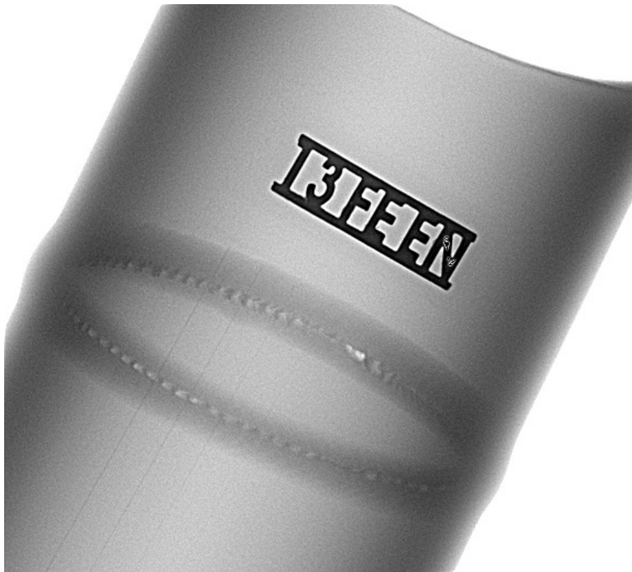
2 x 3 mm thick – 3 inches diameter Fe pipe 135 kV – 1.2 mA – 30s – 90 s with DeReO WA-P 200 \mu\text{m} IQI W16 (100 \mu\text{m} – 1.7 %) / W17 (80 \mu\text{m} – 1.3 %) is resolved
