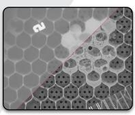
Radiography/ Radioscopy Combine digital radiography and radioscopy with a fantastic sensitivity, excellent signal to noise ratio (SNR) and unbeatable contrast sensitivity better than 1% (EN 462-1). Switch from video to radiography mode during the X-ray shot with automatic and fast averaging.
